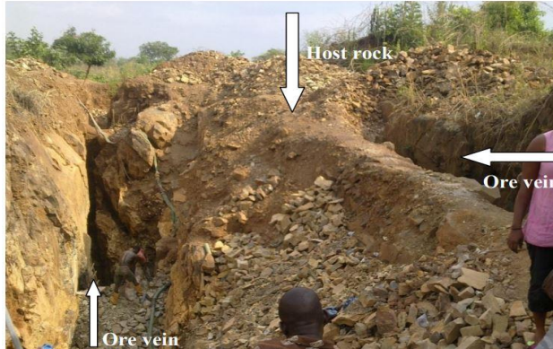
Plate 1: Showing ore vein and surrounding rock exposed by Artisanal mined Pb-Zn vein cutting across the intrusive
