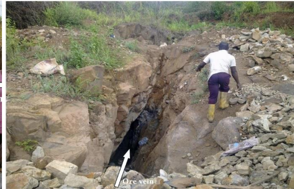
Plate 1: Showing ore vein and surrounding rock exposed by Artisanal mined Pb-Zn vein cutting across the intrusive
