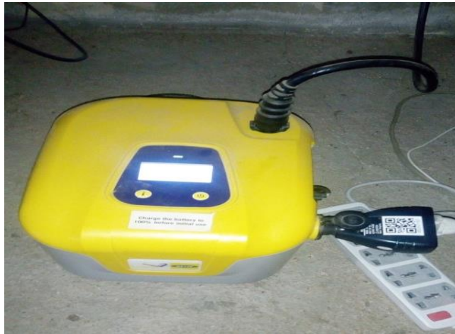
Plate 4: Showing the MTN Lumos box with an inverter that convert dc current to ac current.
