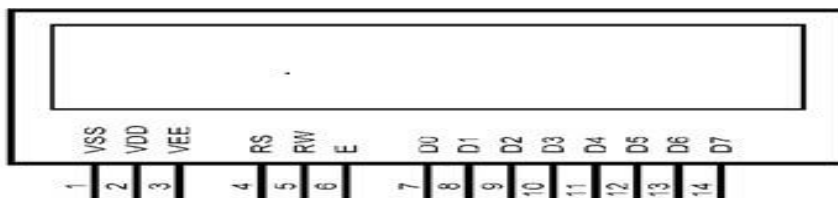
Figure 8: Pin configuration of the 16x2 matrix LCD
